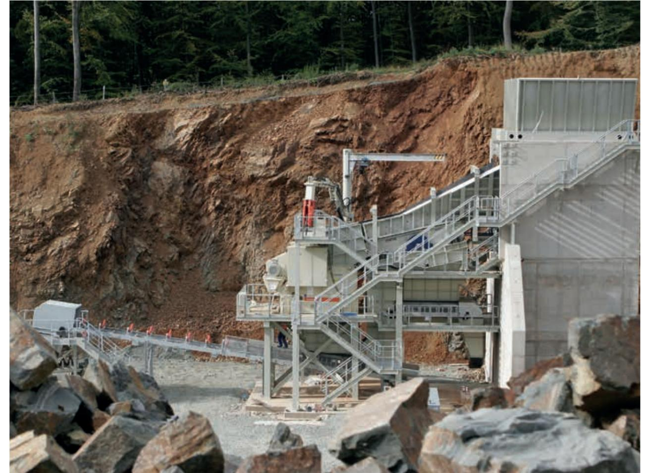
BASIC Vorbrechanlage, Diabase, 500t/h, HAVER F-CLASS, HAVER Schubwagen, Backenbrecher
