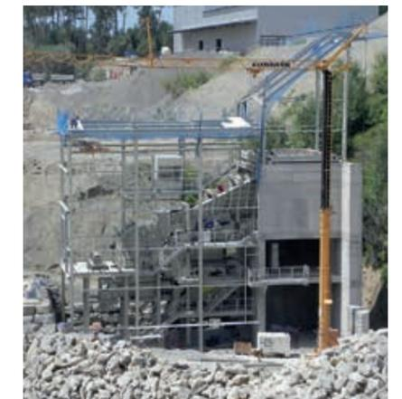
MASTER Vorbrechanlage, Kalkstein, 600t/h, HAVER F-CLASS, HAVER Schubwagen, Prallbrecher
