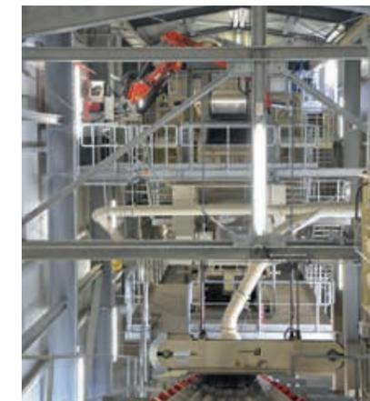
Vorbrechanlage, Rohgips, 400t/h, HAVER F-CLASS, Plattenband, Backenbrecher
