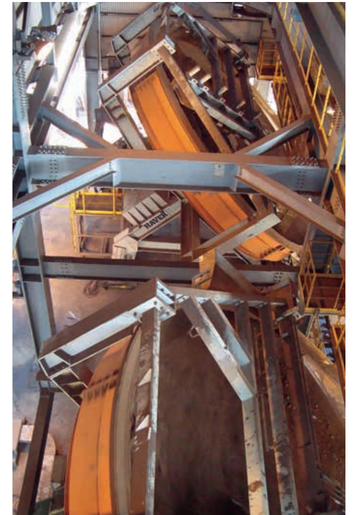
Pelletieranlage, Eisenerz, 140t/h, HAYER SCARABAEUS
