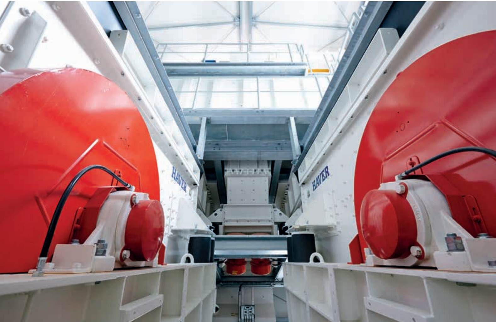
Vorbrechanlage, Grauwacke, 750t/h, HAYER F-CLASS, HAYER Schubwagen, Backenbrecher
