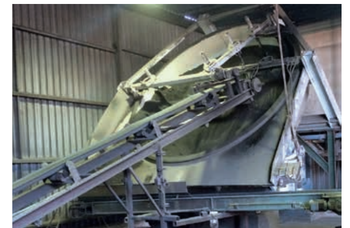
Pelletieranlage, Mineraldünger, 20t/h, HAYER SCARABAEUS
