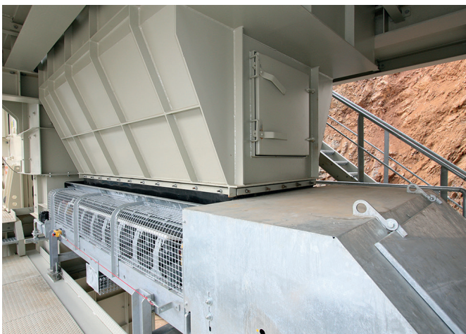
Maintenance-friendly hopper above belt conveyor
