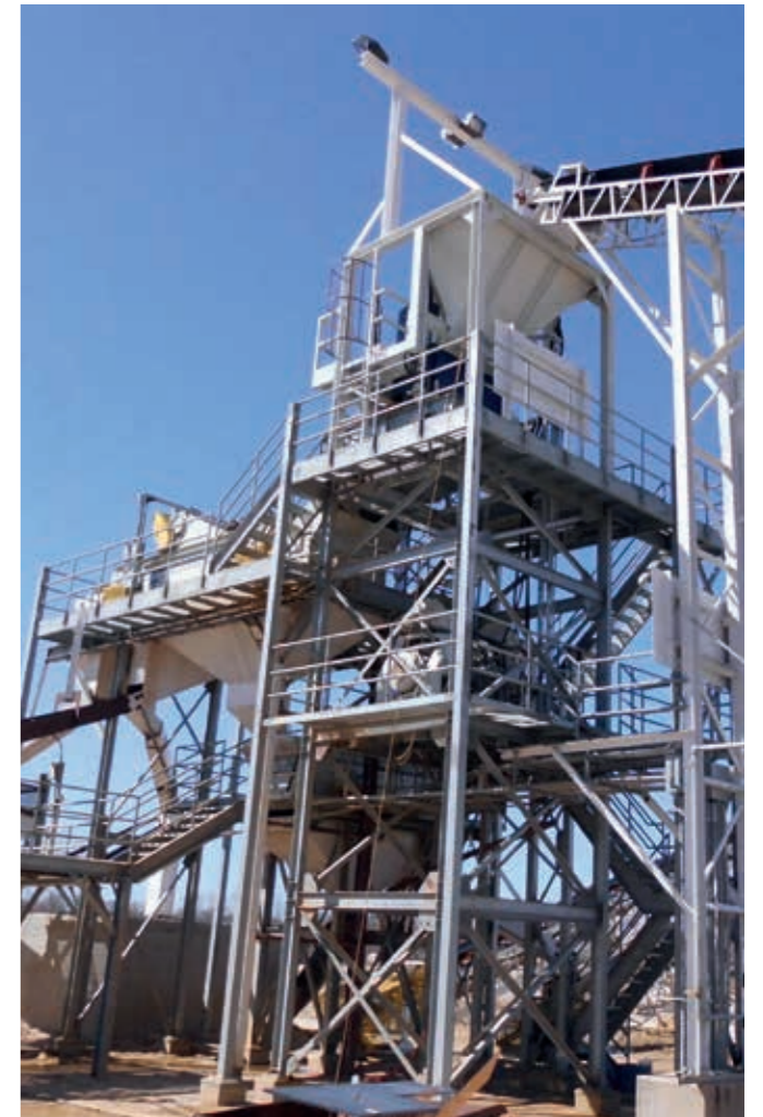
Washing plant, several aggregates, 300t/h, HAVER HYDRO-CLEAN, HAVER L-CLASS
