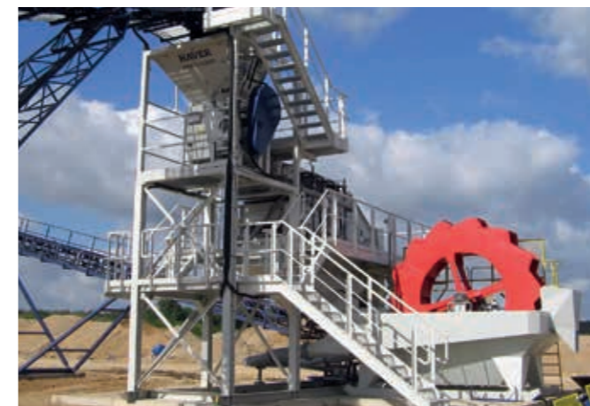
Washing and classifying plant, natural sand, 70t/h, HAVER HYDRO-CLEAN, HAVER L-CLASS, HAVER bucket wheel
