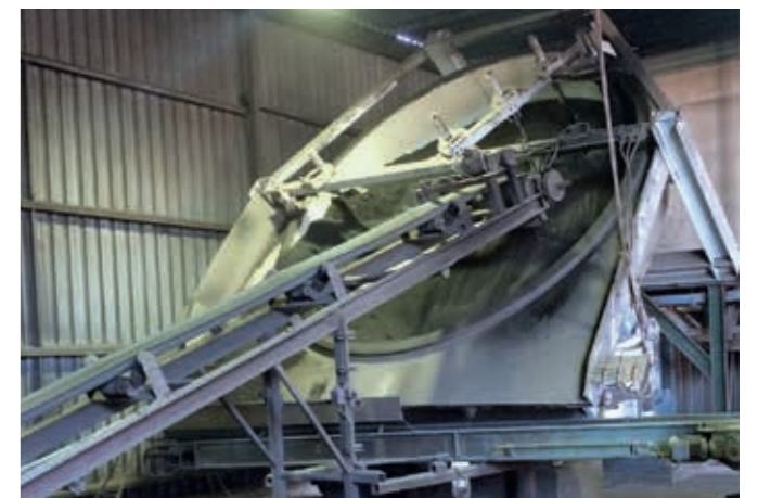
Pelletizing plant, mineral fertilizer, 20t/h, HAVER SCARABAEUS
