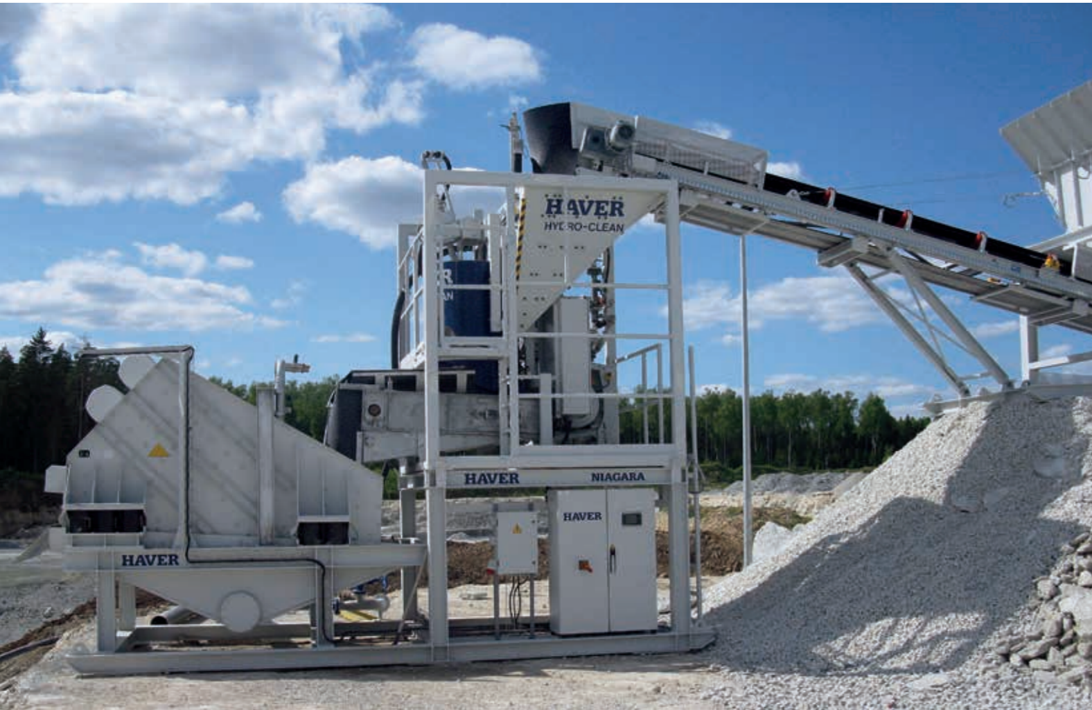
Washing plant, limestone, 70t/h, HAVER HYDRO-CLEAN, HAVER L-CLASS
